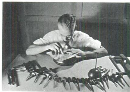
ENGRAVING. Copper-plate and steel-die engraving is a painstaking hand operation requiring years of experience on the artist's part. Few men are engaged in this specialized profession today. ABOVE, the veteran engraver at A. Carlisle & Co., surrounded by an array of cutting implements, engraves a copper diploma plate. BELOW, the steel-die stamping press in operation.
